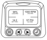
When the diagnostic display receives a severe fault code from an engine control unit the single or four parameter screen will be replaced with the "Shutdown" message.
